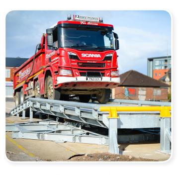
The turntable platform rotates 180-degrees to align with the ramps, to allow the vehicle to drive off in a forward gear. At only 3kW to rotate 32 tonnes and require a standard 32amp 415v supply, the turntable is relatively low power.
