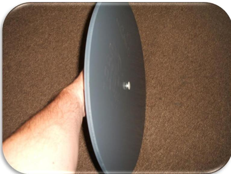
3) Make sure the outer faces of the plastic discs are clean and free from grease and moisture, otherwise the glue may not stick fully – Remove the mat from the rubber mat and centralise over the plastic disc. Apply the mat to the plastic disc, make sure any air bubbles are removed from the mat to the plastic disc. Repeat the process for the other side of the mat. Leave the unit for 24 hours in ambient conditions.
