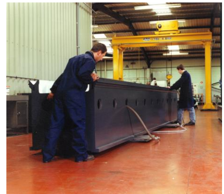
Finished machine beds are moved through a factory on Hovair AL22 air skates
