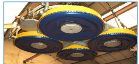
Bottom Right: 5,000kg Carding machines are moved through an assembly flow line on Hovair AS18 air skates
