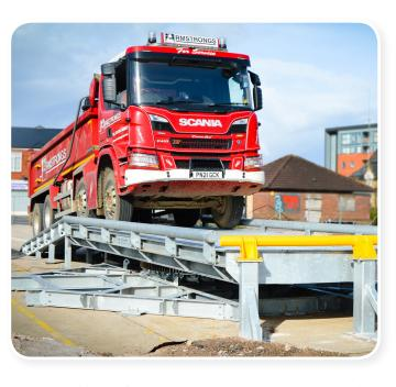
The turntable platform rotates 180-degrees to align with the ramps, to allow the vehicle to drive off in a forward gear. At only 3kW to rotate 32 tonnes and require a standard 32amp 415v supply, the turntable is relatively low power.
