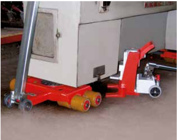
Castors with ball bearings guarantee easy movement.
